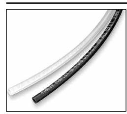
Series NR semi-rigid nylon tubing offers better chemical resistance than series N, good resistance to high ambient temperature and low moisture absorption. NR has a high tensile strength which will give excellent coupling retention in high pressure, temperature and vibration environments.
