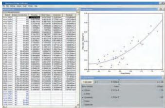
The combinatorial calibration method is particularly powerful because it is not necessary to know the actual values of the four resistors, or their frequency dependence. This means we can calibrate any ac or dc bridge to any accuracy, so long as the various resistance combinations are accurate.
