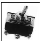
MINIATURE FLAT TOGGLE SWITCH SERIES Specially designed for decorative appearance with ease in smooth switching operation in mind. Specify part number. Specifications Contact rating: 6 Amp–125 Vac, 3 Amp–250 Vac. Bushing: <sup>1</sup>/<sub>4</sub>". Thread length: <sup>5</sup>/<sub>16</sub>". All necessary mounting hardware included.
