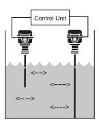
For many applications, water is the liquid being sensed. Raw or tap water usually has naturally occurring salts, chlorides and minerals that make it conductive enough to operate the control. Condensate receiver and cooling tower water are also very conductive due to evaporation. Ultrapure water (RO, deionized, demineralized, etc.) is highly resistive and is not able to conduct the current needed to operate the control.
