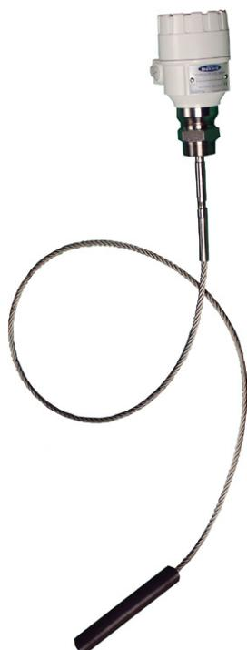
**DESCRIPTION** The TDR-2000 provides continuous, non-mechanical level measurement, utilizing guided wave radar technology. The TDR-2000 is particularly suited for measuring the level of solids, granules, and powders, as well as a wide range of liquids. For many applications, the TDR-2000 is an economical and superior alternative to capacitance, ultrasonic, and plumb bob technologies.
