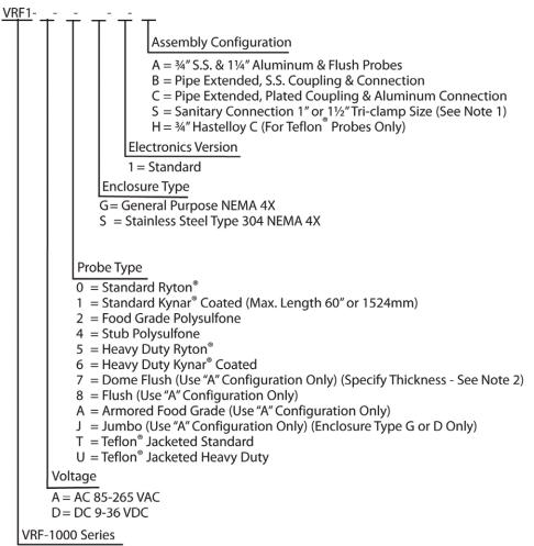
Note 1: For 3A Sanitary Certification add "3A" at end of the model code. Configuration "S" must be used and either "Type 2" Food Grade probe or "Type 4" Stub probe.
