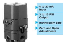
The TA901 Electropneumatic (I/P) Transducer converts a milliamp current signal to a linearly proportional pneumatic output pressure. This transducer is designed for control applications that require a high degree of reliability and repeatability. The TA901 is used in the control operation of valve actuators and pneumatic valve positioners in the petrochemical, HVAC, energy management, textile, paper, and food & drug industries.
