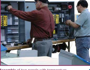
**Assembly** of two panels with temperature controllers and motor drives. Also includes Programmable Logic Controllers (PLC) with communication capabilities pre-programmed by our engineers.
