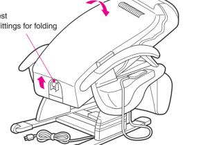
As shown in the figure, Back pad raise the back pad and make sure that the cover of the main body is not torn. Fabric of the main body Main body of the backrest Before using, please raise the back pad to ensure that there is no tear in the fabric or cover. Also, check the chair cover of the other parts
