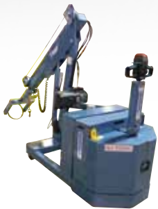
Full Power Custom • Custom full power unit has custom end effector.
