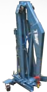
Fold-Up Ruger • Straddle style design • Folds-up for compact storage • Telescopic boom • Fits through standard doorways
