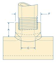
Coupolet<sup>™</sup> fittings are for use in fire protection sprinkler systems and other low pressure piping systems.
