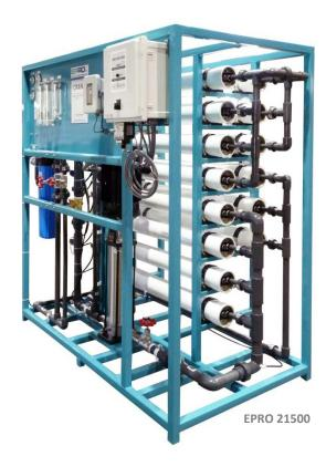
**Electronic control functions include:** low pressure shut down, low pressure auto restart, shut down on high storage tank, pretreatment shut down, system indicator lights- run, low pressure, storage tank full, and permeate TDS sensor.
