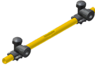
2. Place By-Pass Saddles onto main
