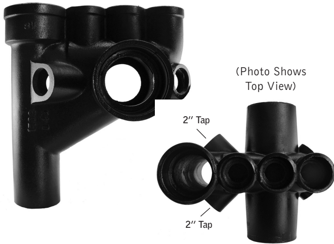
PART NO. SV 1739D Vented Closet Cross with 2" 45° Taps (Designed for use above the floor)
