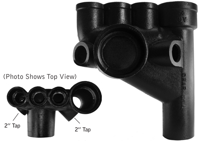
PART NO. SV 1739L Left Hand Vented Closet Tee with 2" 45° Taps (Designed for use above the floor)
