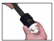
Stab pipe completely into fitting so that the mark on the pipe is within 1/8" from the fitting entrance.
