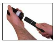
Chamfer end of pipe using Continental's ID chamfering tool with ID gauge.
