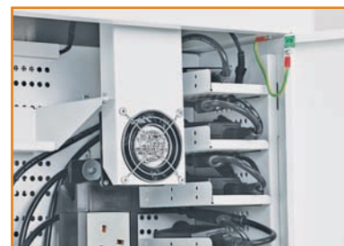
2 x built-in fans provide automatic thermostatic temperature control
