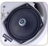
Each Commercial Design model is a true coaxial loudspeaker, with a compression driver concentrically located so that the high frequencies emerge through the center of the low-frequency driver's magnetic structure and cone via a precisely contoured Tru-Phase<sup>TM</sup> HF Waveguilde. This special construction provides consistent, wide dispersion up to 16 kHz.
