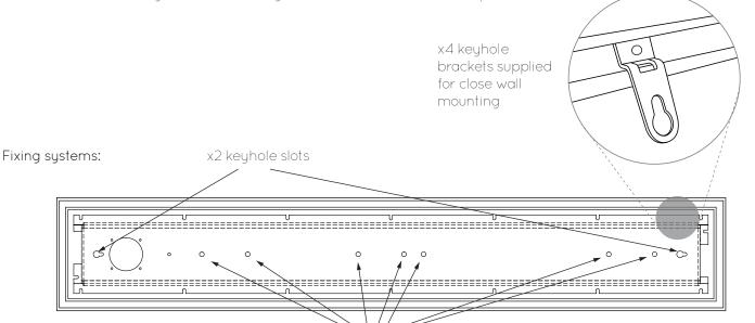
x7 M5 threaded inserts for use with Amina HDWB or other wall brackets (not supplied)
