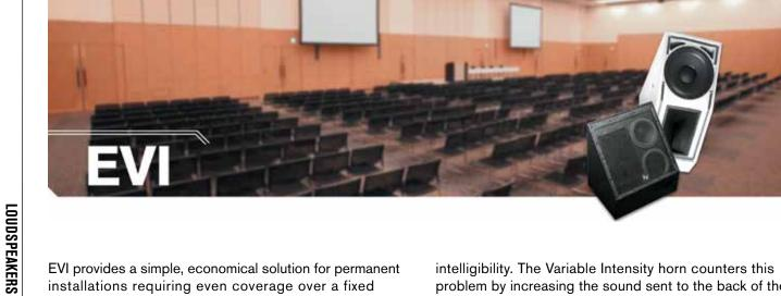
EVI provides a simple, economical solution for permanent installations requiring even coverage over a fixed rectangular area. In a typical room, the distance from a front-mounted loudspeaker to the last row is two or more times the distance to the front row, resulting in a substantial front-to-back difference in level and
