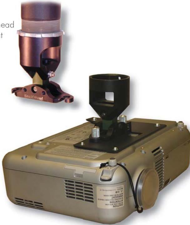
Our "Knucklehead" mount is a superior ball joint design which allows independent adjustment of pitch and tilt axis. The interface plate is custom designed to fit your specific projector chassis, providing full access for lamp changes and filter cleaning. Accommodates most projectors up to 40 lbs.
