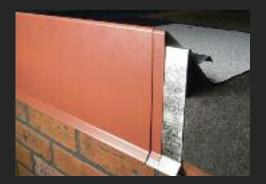
assembly together. Grips the roofing plies without the need for exposed fasteners. Standard face sizes are 6.25", 7.75", 9.25" and 10.75". Custom sizes available upon request. UL Classified to meet the ANSI/SPRI ES-1 Roof Edge Standard.
