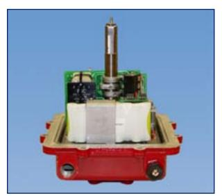
The Quarter master Protek failsafe electric actuator features a rechargeable battery pack, a built-in trickle charger, a low battery indicator, and an auxiliary limit switch that is calibrated with the fail position. The battery pack is installed inside of the actuator housing, so a separate enclosure to house the battery in not required.
