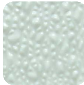
ArmorTuf-NXT with a resin rich surface
