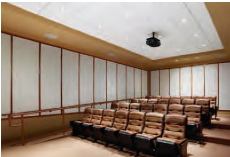
Custom Soundsoak Wall System in Custom Carnegie Strie fabric with Kerf edge detail
