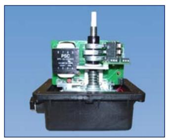
The Quarter Master Protek Failsafe electric actuator features a rechargeable battery pack a built-in trickle charger, a low battery indicator, and an auxiliary limit switch that is calibrated with the fail position. The battery pack is installed inside of the actuator housing, so a separate enclosure to house the battery in not required.
