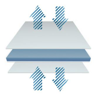
PCM, or Phase-Change Material, is a substance with a high heat of fusion which, melting and solidifying at a certain temperature, is capable of storing and releasing large amounts of energy. Heat is absorbed or released when the material changes from solid to liquid and vice versa; thus, PCMs are classified as latent heat storage (LHS) units.
