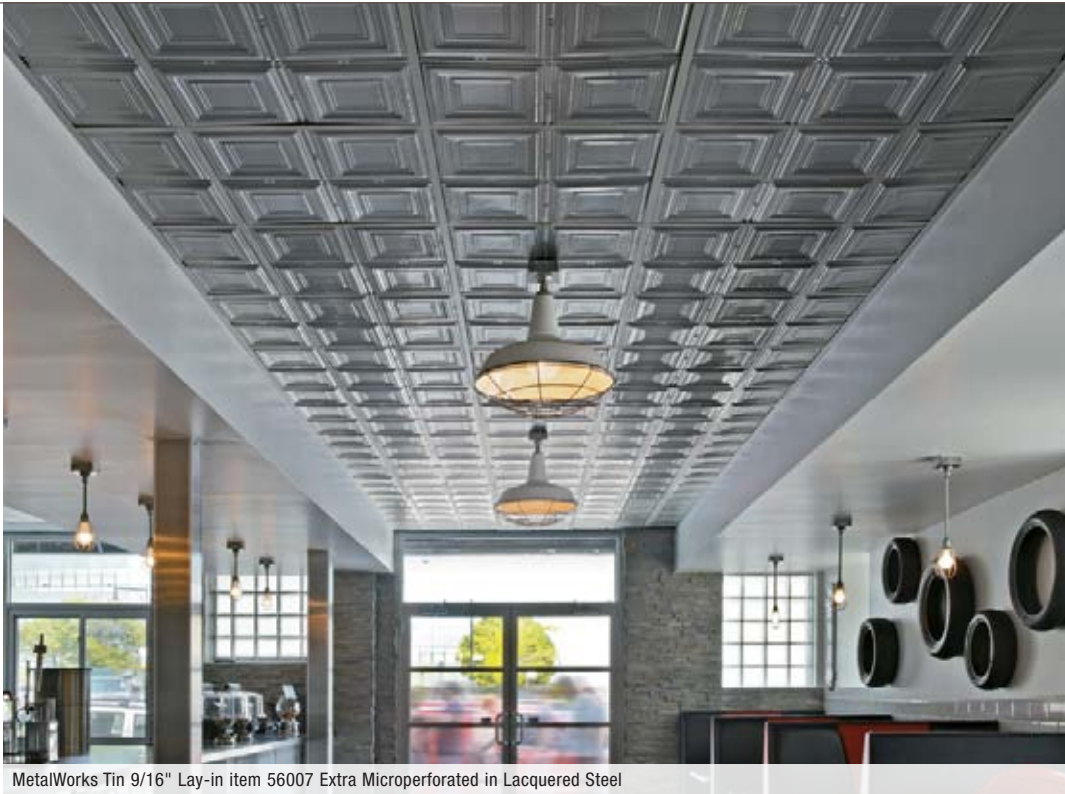
MetalWorks Tin 9/16" Lay-in item 56007 Extra Microperforated in Lacquered Steel
