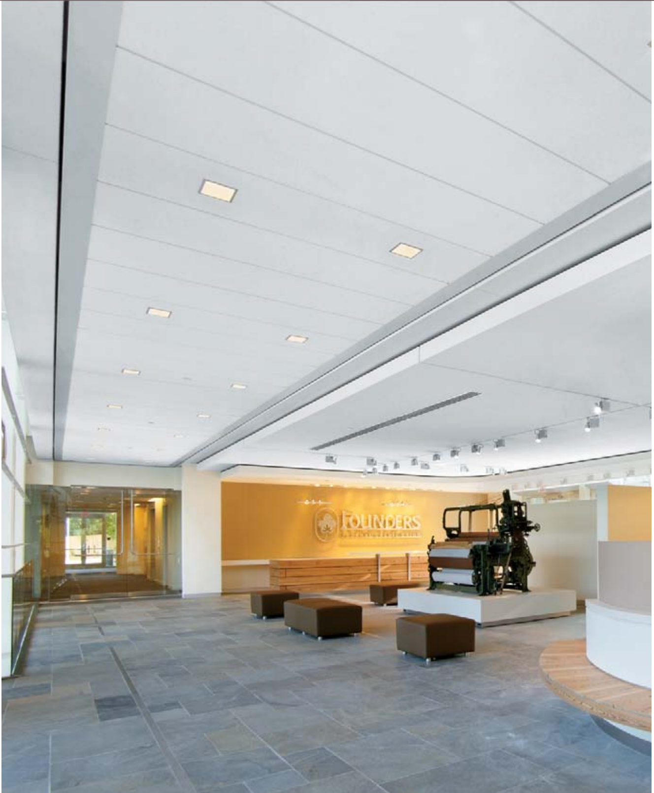
Optima® Vector® Plank 24" x 96"; Prelude® XL® 15/16" suspension system; Axiom® Building Perimeter System
