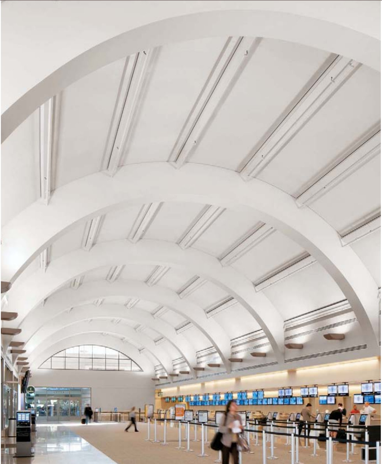
MetalWorks™ Torsion Spring Custom Curved Ceiling System 30" x 82" planks with Rg 2516 perforation in Cream Weave finish
