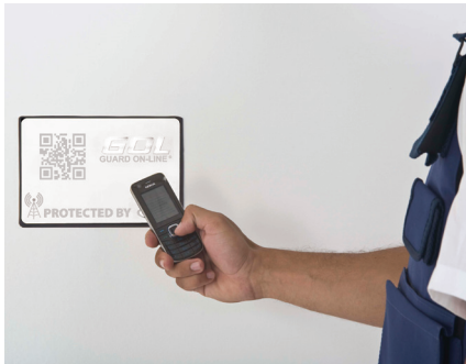
The patrol officer uses the mobile device in place of a tour verification device. An image of the QR code is taken by the camera on the mobile device and GOL-QR sends the tour information immediately to Guard On-Line
