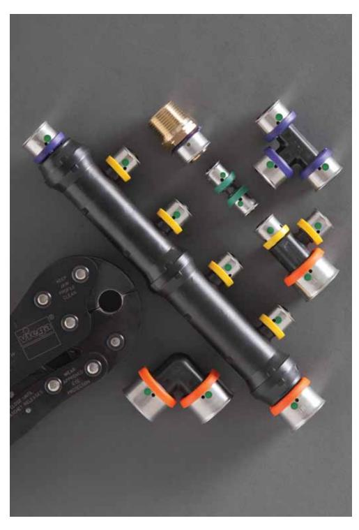
Viega's new PEX Press polymer fittings help installers save time on the job so they can accomplish more. This fitting system provides 40 percent less pressure drop compared to standard U.S. polymer PEX crimp insert fittings. The only PEX fitting in the industry with the Viega Smart Connect® leakdetection feature, Viega PEX Press polymer fittings are made in the U.S.A. and are approved for potable water and radiant applications in residential and light commercial projects.
