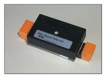
Module **RRU** is a unit which can be connected to the **CEIA** Metal Detectors by means of the top and bottom communication port, used for repeating the detection alarms of the gate through a relay.
