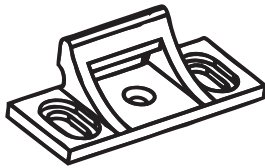
97 Top Surface - non-roller top strike for 20/21 Series Surface Vertical Rod Devices
