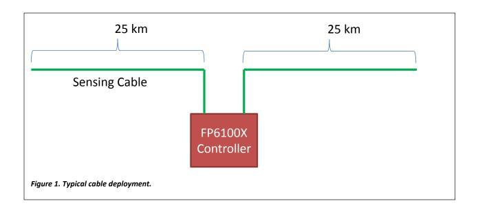
2. **Fiber optic sensor cable**, buried along with the pipeline. The cable is an armored, multi-fiber, single mode, telecommunications-type of cable suitable for direct burial. Standard cable deployment for third party interference detection purposes for the FP6100X is directly above the buried pipeline, at a depth approximately 20-30 cm (8-12") above the pipeline. The recommended cable deployment is shown in Figure below.
