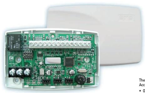
The 734 Wiegand Interface Module allows you to add Access control capability to any DMP Panel.
