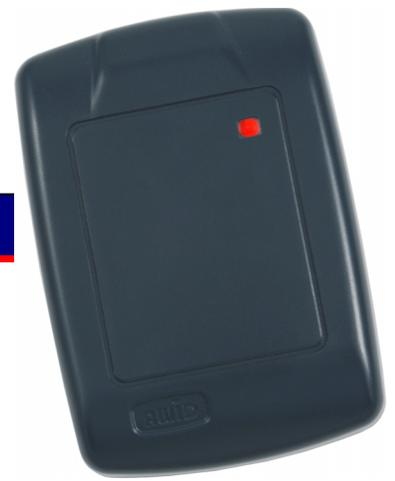
AWID's UA-612 UHF Access Reader is a combination of UHF generator, reader electronics, and transmit/receive antenna in a single small, attractive switchplate-type enclosure. It is easily installed on an electrical box or wall, with simple wiring like a proximity reader. The enclosure is a modern, sleek design using molded ABS engineering plastic with a deep black color.
