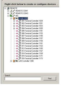
The X-LAN is an Ethernet to RS-485 converter that bridges the gap between two industry standard networks.
