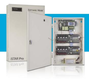
iSTAR Pro is an intelligent, modular controller that offers a cost-effective access control solution for up to 16 doors. It features onboard Ethernet, embedded intrusion zone functionality, peer-to-peer communication, local/global anti-passback control, and up to 128 MB memory – enough to store over 500,000 cardholders.
