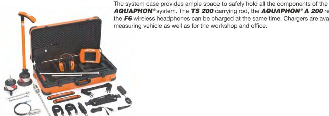
AQUAPHON® system. The TS 200 carrying rod, the AQUAPHON® A 200 receiver and the F6 wireless headphones can be charged at the same time. Chargers are available for the measuring vehicle as well as for the workshop and office.
