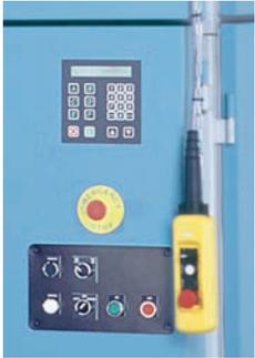
The controls are composed of two (2) basic sections: the drying controls and the load/unload controls.
