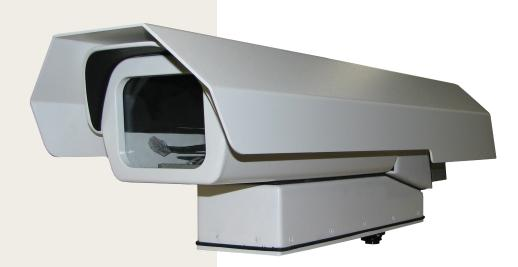
The Thermo-Electric Cooled (TEC) Housing was designed to provide a safer solution for IP cameras installed in high ambient temperature environments. Typically, IP cameras generate a large amount of heat during normal operation. Excessive heat can cause temporary or permanent damage to the camera. When installed in high temperature environments, the heat from the camera combines with the heat of the environment and can threaten camera failure.
