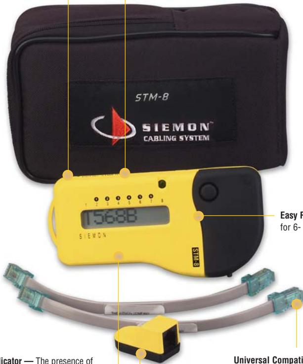
**Line Voltage Indicator** — The presence of line voltage is indicated on the display to help prevent accidental damage to the unit
