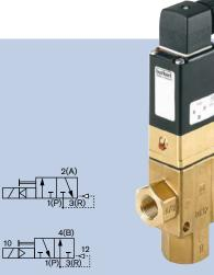
The pilot-controlled 3/2-way valve, Type 0344, with a smoothly operating servo-piston requires a differential pressure of 0.25 bar for complete opening and closing. In the circuit functions NC and NO, it is particularly suited for use with neutral gases with low pressures and for vacuum, even with dry running.
