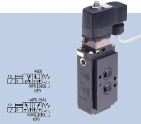
Type 6519 NAMUR Ex m/me valve for process plants switches reliably, even when fully restricted. The valve made out of premium polyamide can be operated either as a 5/2 or a 3/2-way version through different mounting plates. The NAMUR flange interface allows easy assembly on different pneumatic actuators on the spot.
