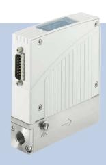
Mass flow meters are used in process technology for the direct measurement of the mass flow of gases. In case of volumetric flow meters, it is necessary to measure the temperature and the pressure either the density, because gases change their density or rather their volume depending on the pressure. The measurement of the mass flow, on the other hand, is independent on pressure and the temperature.
