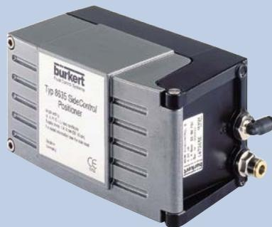
The SideControl Positioner, Type 8635, is an electropneumatic positioner for pneumatically actuated process valves with linear or part-turn actuators. It is excuted in two conductor technology. Signal processing, control and actuation of the internal positioning system are accomplished with microprocessor-controlled electronics. The software function Autotune implemented therein enables automatic adaptation of the positioner to the control valve in use.
