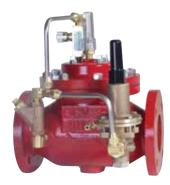
The model 108FPS is used to prevent the fire pump from outdrawing the available supply. In so doing, it protects the pump suction supply from damage associated with a pressure that is too low or backflow and assures adequate supply pressure to the fire system components. **FEATURES:**
