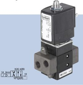
Type 5420 is a pilot-controlled 4-way seat valve with servo-diaphragms. A minimum differential pressure of 2.5 bar is needed for switch-over. The valve can be mounted on two-channel manifolds with a common pressure
