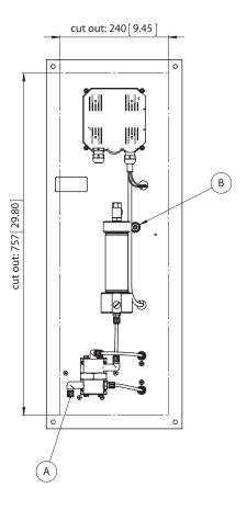
A: Sample inlet PE tube Ø4x6 mm or Ø1/6"x1/4" (US version)  $5^\circ$  to  $45^\circ$ C (40° to 115°F), pressure 0.5 to 6 bar (7 to 90 PSI), flow 12L/h
