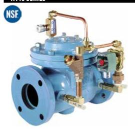
The Apollo Series A115 Solenoid Control Valve is designed to provide on/off or open/close control of fluids in response to an electrical signal. The valve consists of the basic Apollo model A65 with solenoid-operated pilot. With the appropriate solenoid, the valve may be normally closed (energize to open) or normally open (energize to close).
