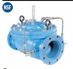
The Apollo Series A94 Check Valve is a simple on-off valve that opens to allow forward flow when inlet pressure exceeds outlet and closes tightly to prevent backflow when outlet pressure exceeds inlet pressure.
