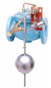
The Apollo Series A800 Float Control Valves are designed to maintain a desired level in a tank or reservoir by opening for filling the tank when fluid is below the high level point and closing tightly when the desired level is reached.
