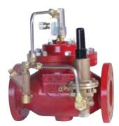
The model 108FPS is used to prevent the fire pump from outdrawing the available supply. In so doing, it protects the pump suction supply from damage associated with a pressure that is too low or backflow and assures adequate supply pressure to the fire system components.
