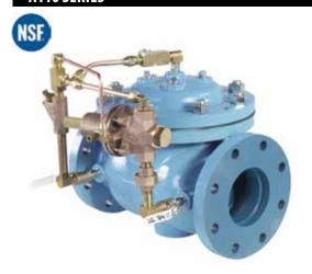
The Apollo A110 Series Differential Control Valve is designed to accurately control the pressure difference between any two points. In some systems this means the valve remains closed until pressure differential commands its opening. It is a pilot operated, modulating type valve which controls pressure accurately and consistently at the desired setting.
