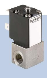
The direct-acting solenoid control valve, Type 2871 (20 mm installation width), is used as the regulating unit in control loops. Due to an elastomeric seat seal the valve closes tight, up to the DN specific nominal
