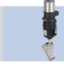
The 2702 Control Valve consists of an 316L angle seat body with a rugged pneumatic piston actuator. The parabolic trim results in a flow characteristic approximately 35% larger than conventional control valves. When combined with the 8692 TopControl, a unique control valve system is formed which can be operated as a simple, accurate positioner for flow rate, temperature or pressure.
